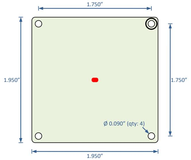
● Approximate location of temperature sensor on bottom side of PCB
